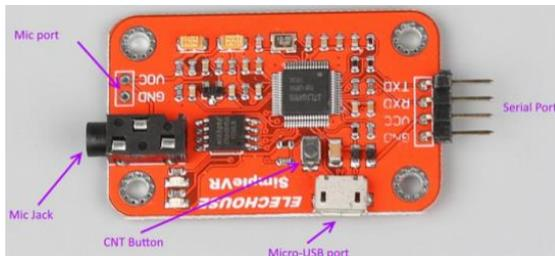
**Figura 3-2:** Voice recognition Module V3
