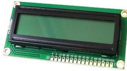
**Figura 16 – 2:** Pantalla LCD 16X2
