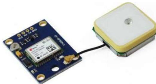
**Figura 15-2:** Sensor GPS NEO – 6M
