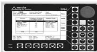
Safety Evaluation mode enables contributions from individual telecom services to be compared with the total field strength value. Here, the results are shown as a percentage of the permissible exposure level.
