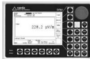
In Time Analysis mode, the SRM measures one peak value or RMS value against time. Changes in the measured values over a period of time can be recorded in this way.
