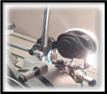
A photograph showing a halogen lamp connected to the alternator. The lamp is mounted on a metal frame and is illuminated, casting a bright light. The setup is part of a laboratory experiment to load the motor.                                                                    |
