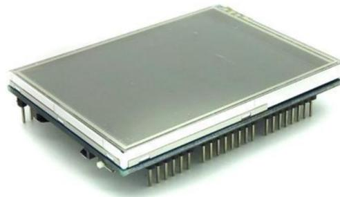
The Arduino 3.2" TFT Touch Mega Shield is designed for all the Arduino Mega compatible boards. It works in 3.3V voltage level. It can be directly plugged on the Arduino Mega and other compatible boards. It will offer display, touch and storage functions for the Arduino Mega board.
