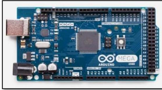
Figura 4-2 Arduino Mega 2560
