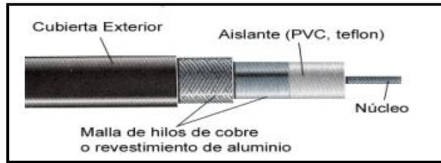
Figura 13-5 Cable coaxial
