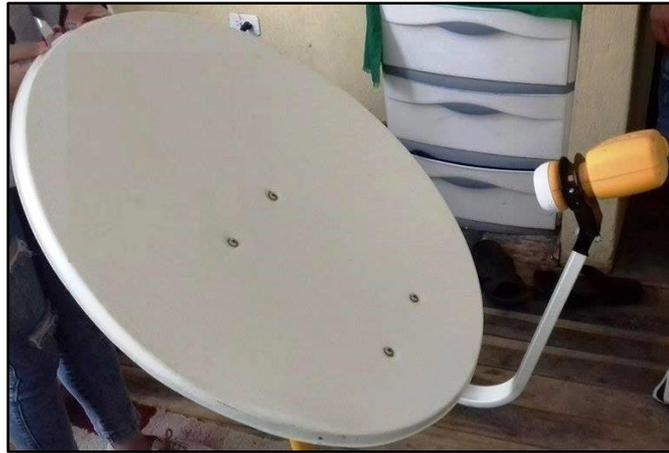
**Figura 4-2** Antena Parabolica Off-Set
