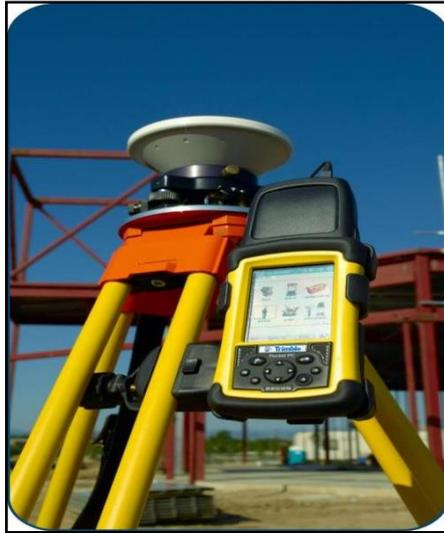
**Figura 3-1.** Receptor GPS
