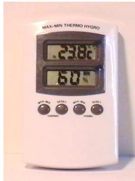
**FIGURA N°8. TERMOHIGRÓMETRO**
