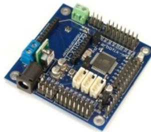
**Figura 5-1:** Arbotix-M Robocontroller.
