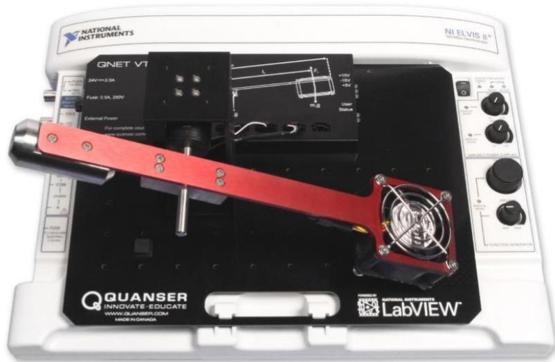
**Figura 5-1 QNET VTOL conectada a NI ELVIS II**
