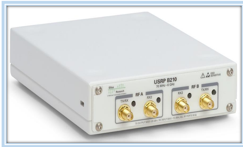
Figura 2-2: Vista frontal d la USRP B210
