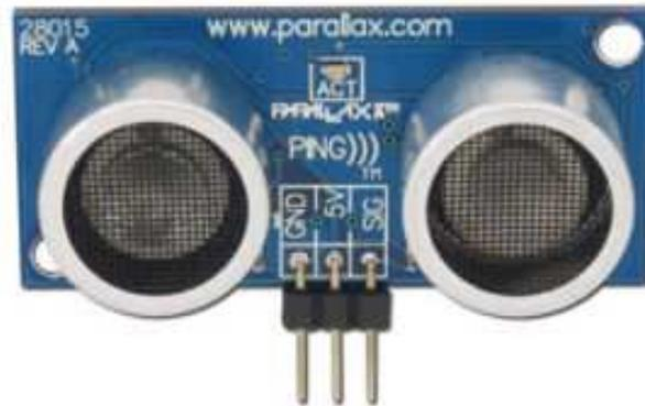
FIGURA IV.2: Sensor Ping Parallax
