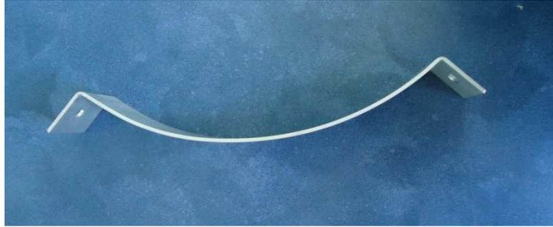
**Fig. V.54 Arco defectuoso**
