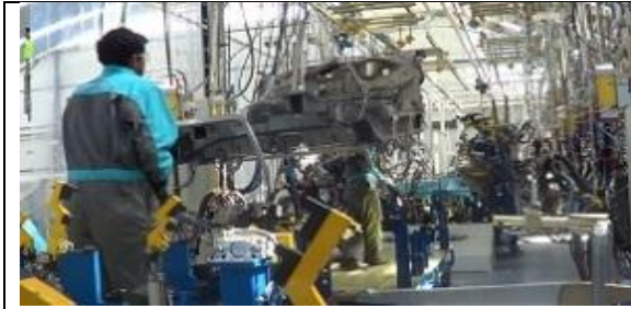
Figura 10-3: Transporte de JIG 1 a JIG 2
