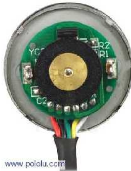
37D mm metal gear motor with 64 CPR encoder.
