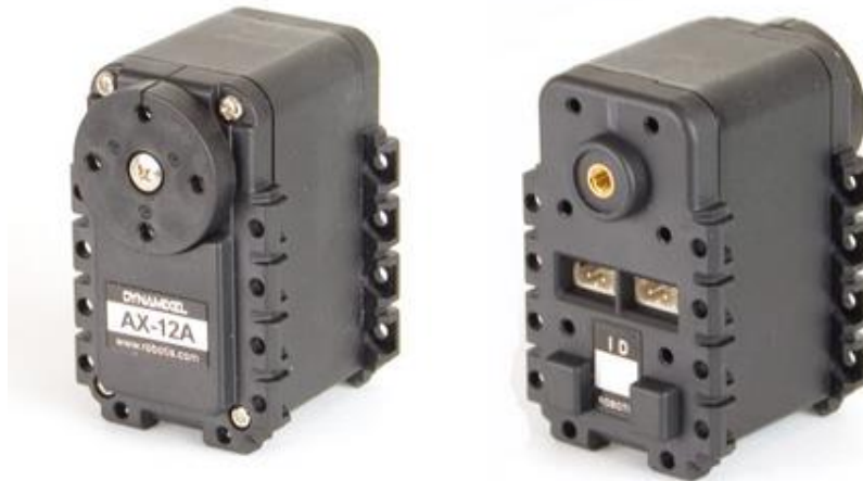
Figura II-20: Servomotor Dynamixel AX-12A.
