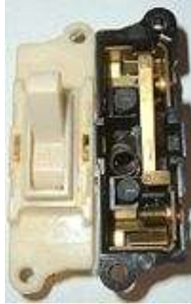
Figura N° II.3. Interruptor sencillo, SPST
