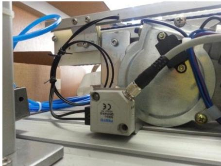
FIGURA. IV.23 SENSOR ÓPTICO FIBRA DE VIDRIO<sup>98</sup>
