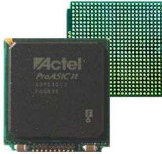
**FIGURA III.4:** CHIP FPGA ACTEL
