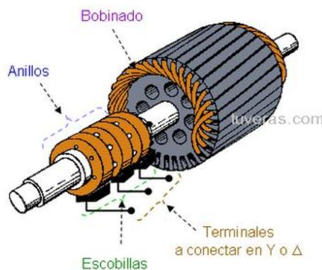
**Figura III-10 Rotor<sup>16</sup>**
