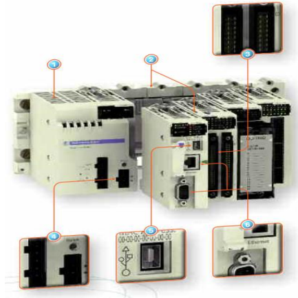
Figura III.29 PLC Telemecanique MODICON M340 35
