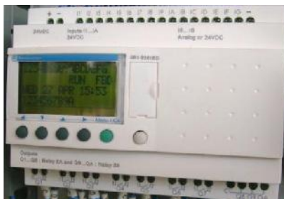
Fig. IV. 2. PLC Zelio Logic
