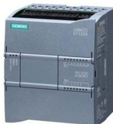
Fig.III.13 PLC Siemens S7-1200
