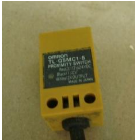
Figura II.23. Sensor OMRON TL-Q5MC1-5
