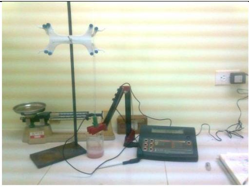
A photograph of a laboratory setup for acidity analysis. The setup includes a metal stand with a white plastic component, a digital scale, a beaker containing a pink liquid, and a digital display unit. The background shows a wall with a power outlet.                                                                                                              |
