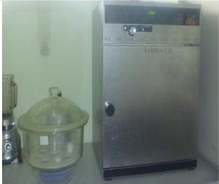
A photograph of a laboratory oven, likely used for moisture analysis. The oven is a tall, stainless steel unit with a digital display and control panel at the top. To the left of the oven, there is a glass desiccator jar with a lid, sitting on a blue base.                                                                                                          |
