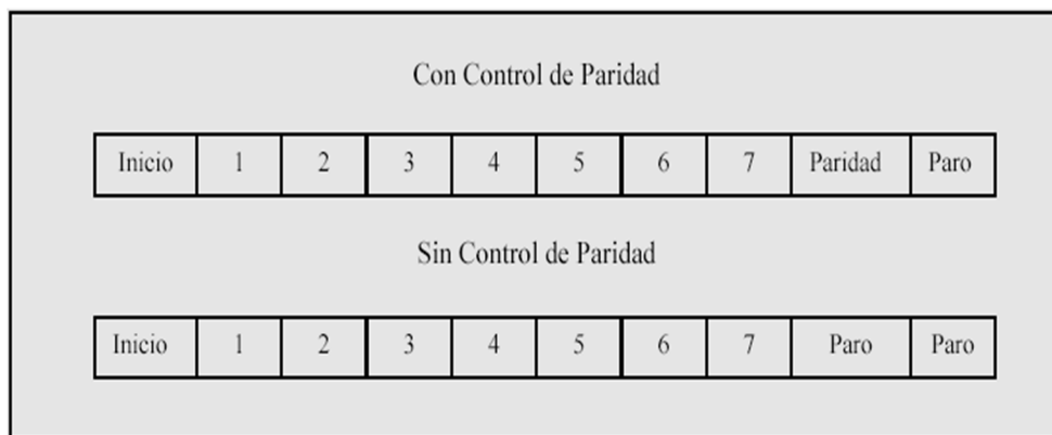
Figura III.9. Orden de bits (ASCII)
