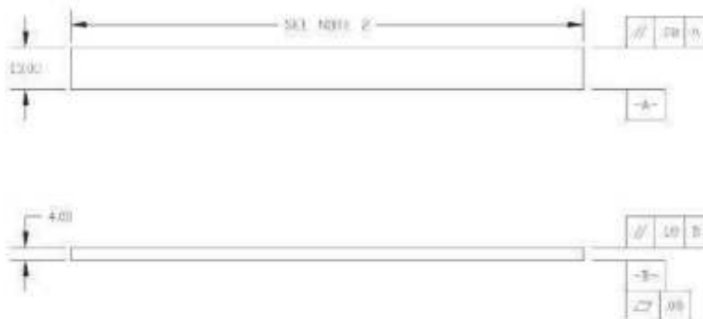
Note: 1—Drawing interpretation per ANSI Y14.5-1999 and ANSI B46.1-1995. Note: 2—See 8.2 and 11.3 of this test standard for the required values of span and overall length. FIG. 4 Standard Flexural Test Specimen Drawing (SI)
