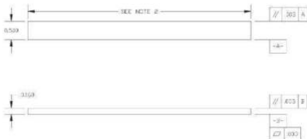
FIG. 5 Standard Flexural Test Specimen Drawing (Inch-Pound)
