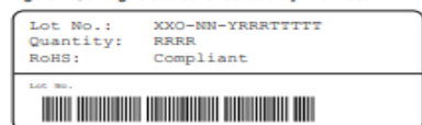
Figure 22: First label on reel: XX = Sensor Type (25 for SHT25), O = Output mode (D = Digital), NN = product revision no., Y = last digit of year, RRR = number of sensors on reel divided by 10 (200 for 2000 units), TTTT = Traceability Code.
