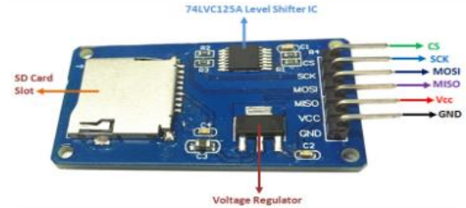
Micro SD Card Adapter Module Pinout
