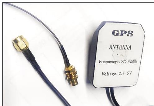
**Figura 7-3:** Antena GPS 1575 4.2MHz
