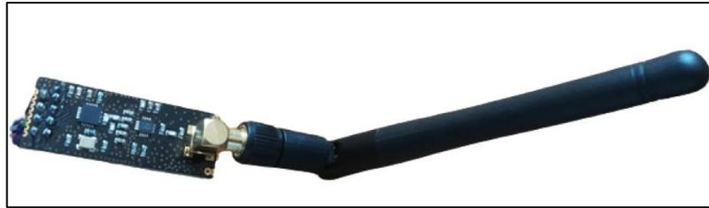
**Figura 8-3:** Antena RF NRF24L01
