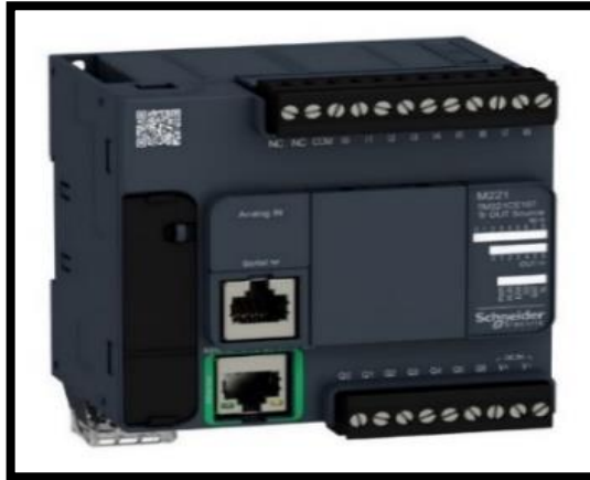
Figura 25-3: PLC Schneider TM221CE16T.
