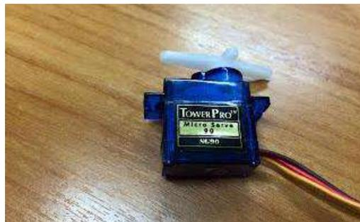
**Figura 22-2:** Servomotor Tower Pro SG-90
