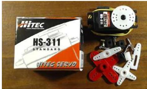
**Figura 21-2:** Servomotor Hitech HS-311
