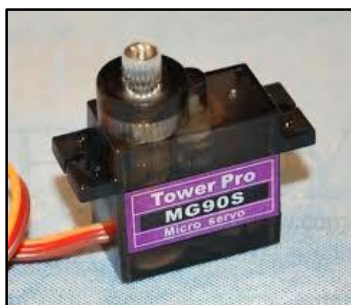
Figura 9-3: Servomotor tower MG90S Realizado por: Castro Carolina, 2022
