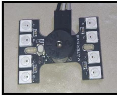
**Figura 15-3:** Led WS2812B & Loud Buzzer.
