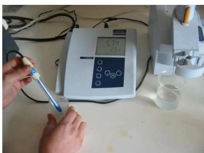
**FOTOGRAFÍA 10. PHMETRO INOLAB WTW**
