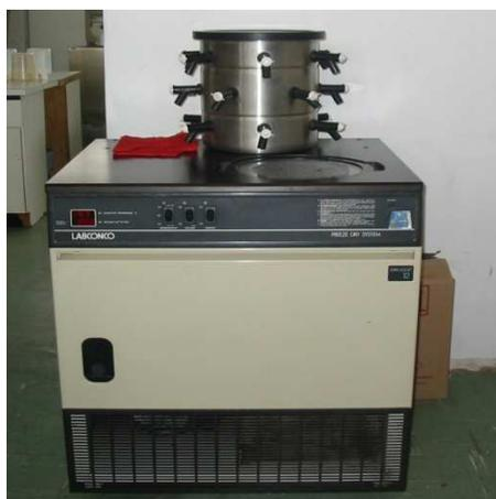
**FOTOGRAFÍA 7. LIOFILIZADOR LABCONCO**
