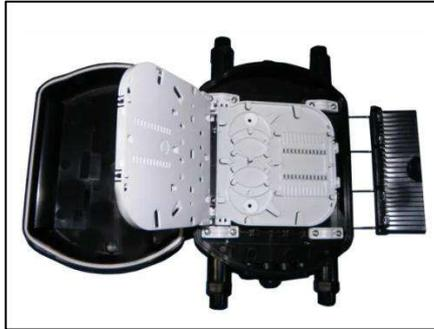
**Figura 30-2:** Caja de empalme Cablix OSCH-12
