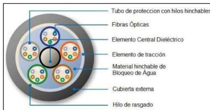
**Figura 10-2:** Cable Loose Tube
