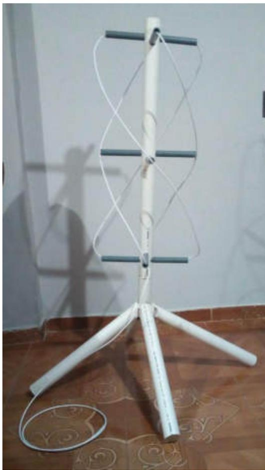
**Figura 36-2:** Antena QHA Balun infinito adherente (Antena 1).
