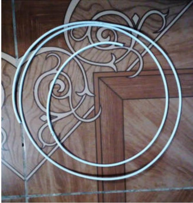
**Figura 31-2:**Espira corta, cable coaxial RG-58 (Antena 1).
