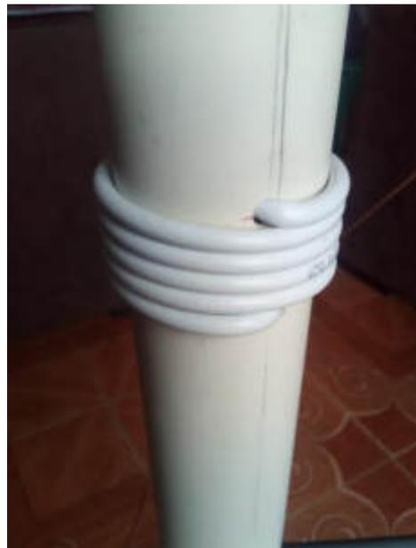
**Figura 41-2:** Inductor de cable coaxial (Antena 2).
