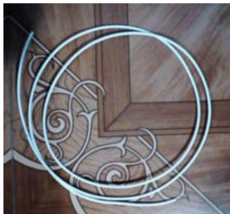
**Figura 30-2:** Espira larga, cable coaxial RG-58 (Antena 1).
