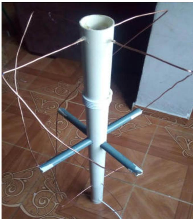
**Figura 42-2:** Antena Cuadrifilar Helicoidal QHA (Antena 2).
