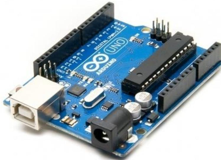
**Figura 30-2.** Tarjeta Arduino UNO R3
