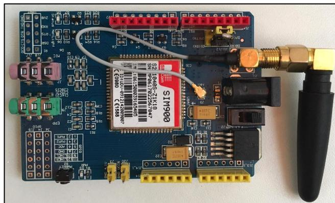
**Figura 9-2:** Tarjeta SIM900 GSM/GPRS
