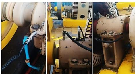
**Figura 4-3:** Horizontal, Vertical y Axial
