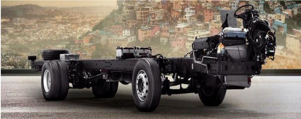
Figura 1-2: Chasis Mercedes-Benz OF-1723/59.
