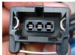
**Figura 3.21** Conector del sensor TPS
