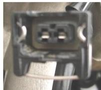
**Figura 3.26** Conector del sensor ECT
