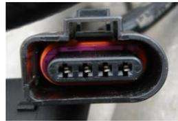
**Figura 3.31** Conector del sensor IAT
