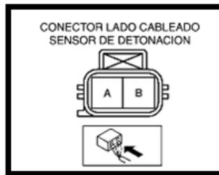
**Figura 4.20** Conector del sensor KS
