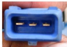
**Figura 3.24** Conector del sensor KS
