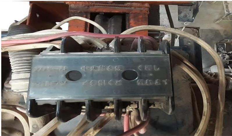
**Figura 35-3.-**Contactor #1 del motor-reductor carro horizontal
