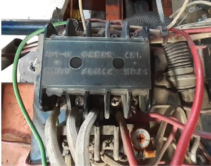
**Figura 37-3.-**Contactor #2 del motor-reductor carro horizontal
