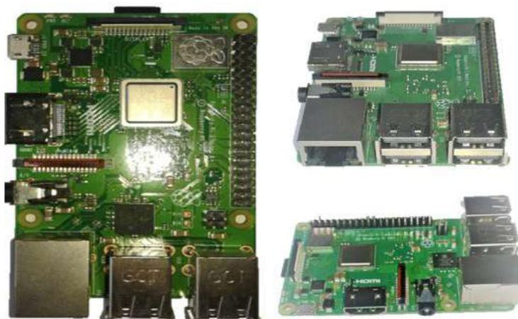
**Figura 5-2:** Raspberry Pi 3 Model B+
