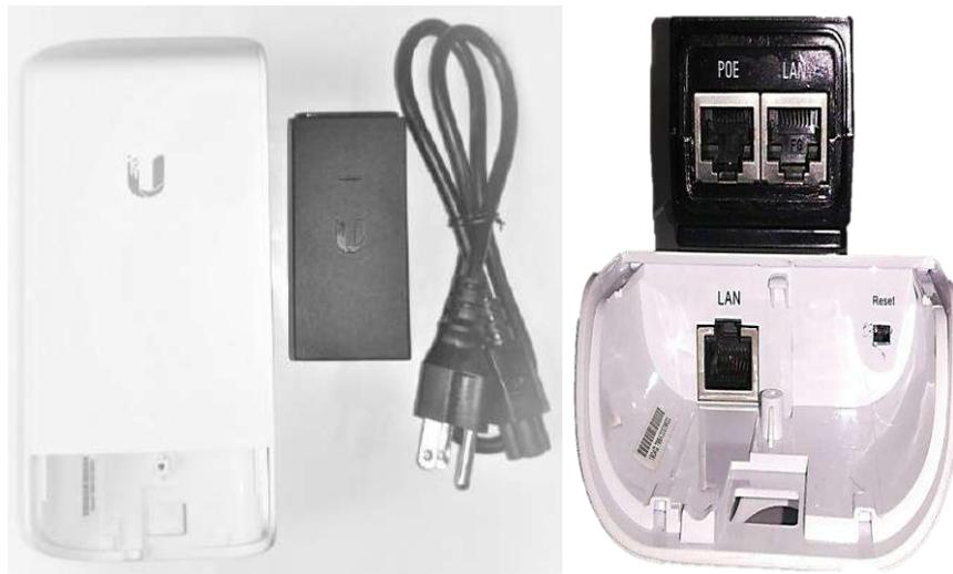
**Figura 6-2:** Antena Ubiquiti NanoStation Loco M2.
