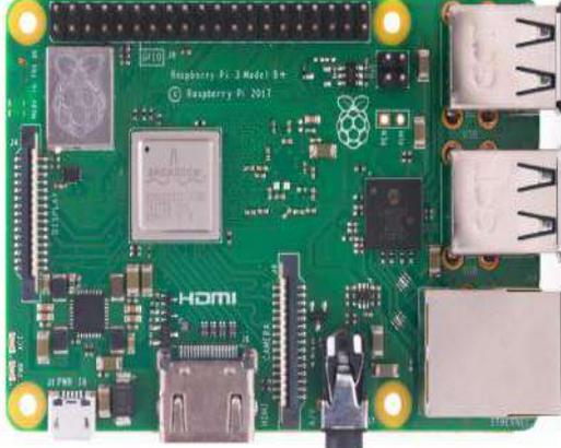
The image shows the Raspberry Pi 3 Model B+ board, a green printed circuit board with various components including a processor, memory, and connectors. The board is labeled 'Raspberry Pi 3 Model B+' and 'Raspberry Pi 2017'.
